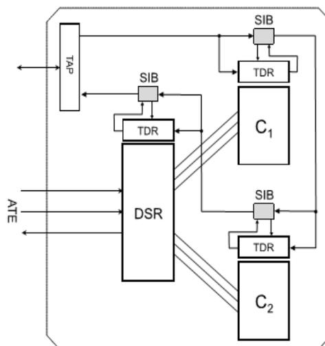
Fig.3. Using IJTAG network to transfer control data
