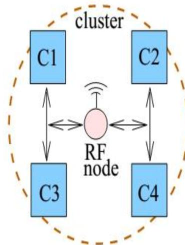
Figure 5: A RF node in a cluster of cores.
