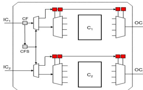
Fig.4. Dedicated control chain-based architecture.
