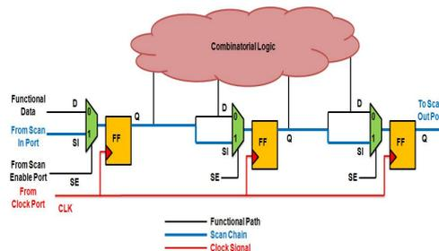
Figure 1.A Typical Scan Chain
